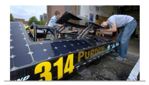
This is a picture of Purdue's solar car. Our car will have this style of hatch - the front of the canopy will swing forward, and the driver will exit to the side in between the two roll cage bars. The hatch materials will be attached to the rollcage, since this is the most sturdy part of the car. The hatch will close with a double sided latch (which is picked out from McMaster) so that both the driver and someone outside of the car will be able to detach the canopy.
