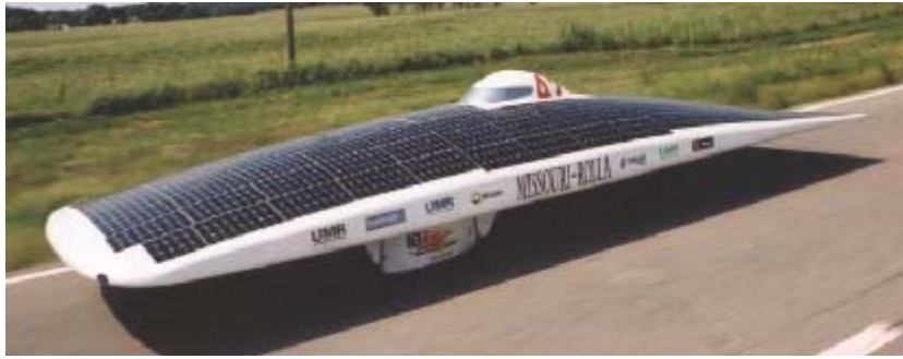
Missouri-Rolla Solar Car, 2003 American Solar Challenge Champion Small Cross-Sectional Area Slightly Curved Underbelly
