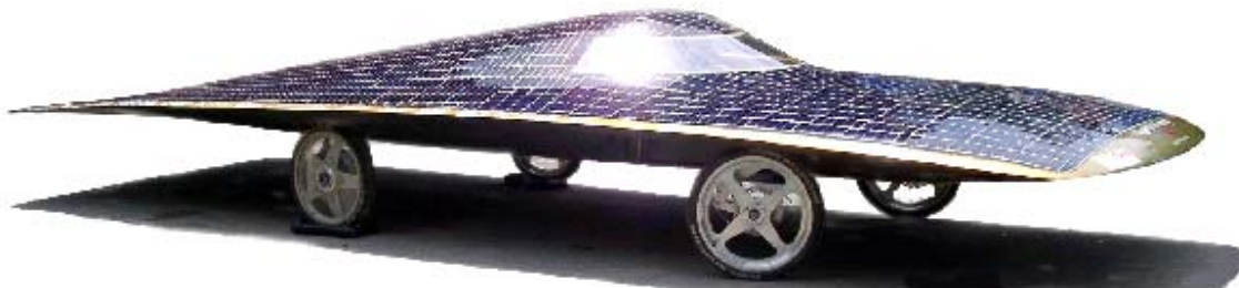
Queens University Solar Car: A slightly curved underbelly Small Cross-Sectional Area Gentle Slope from back of Canopy to back of Car
